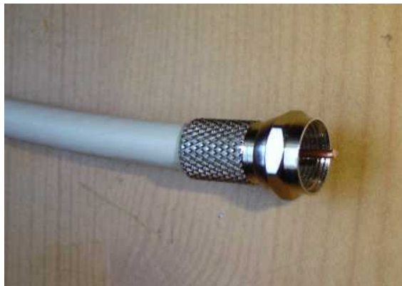
One of the most common types of transmission line, coaxial cable.
